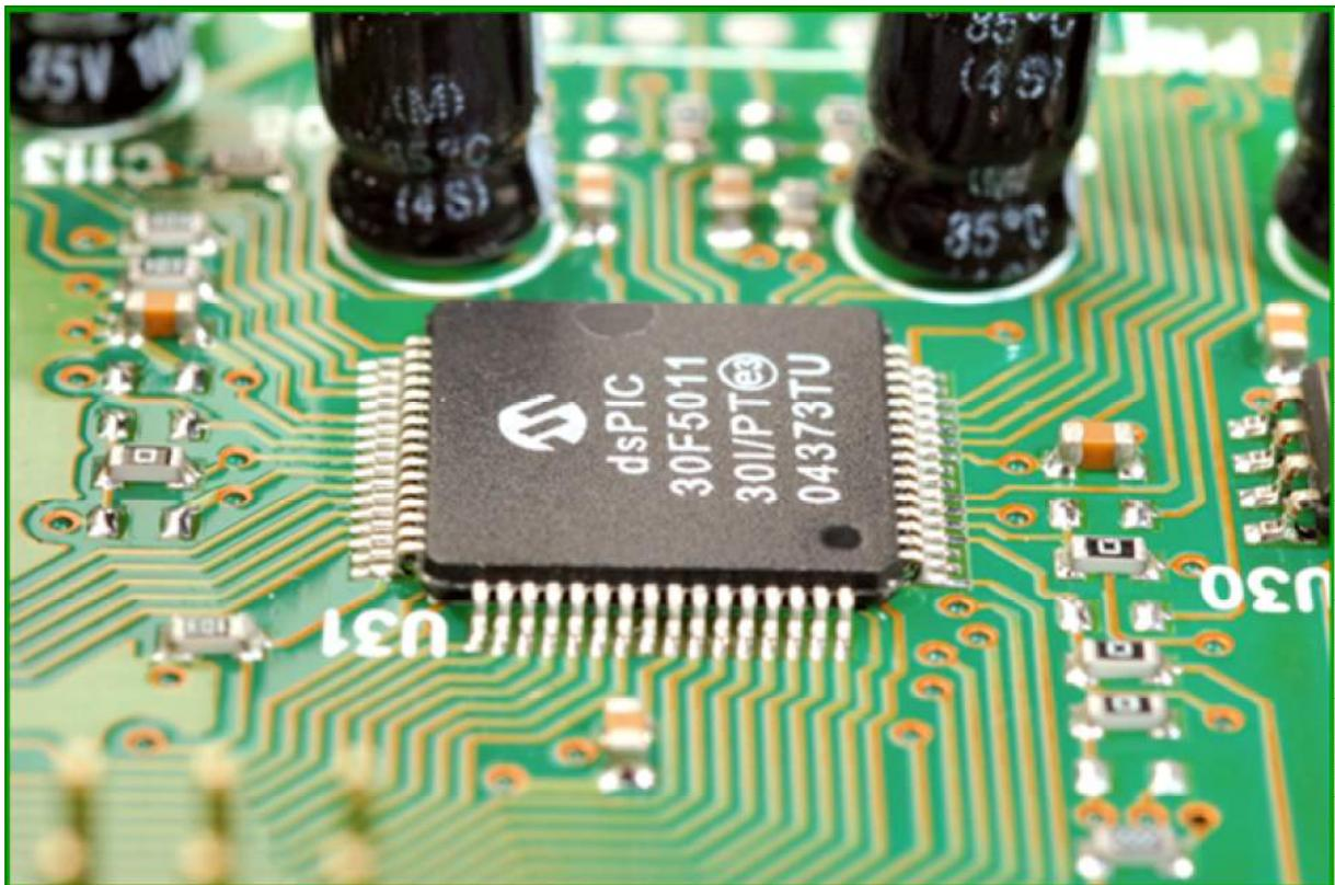
*Detail of the microprocessor on the control card*
